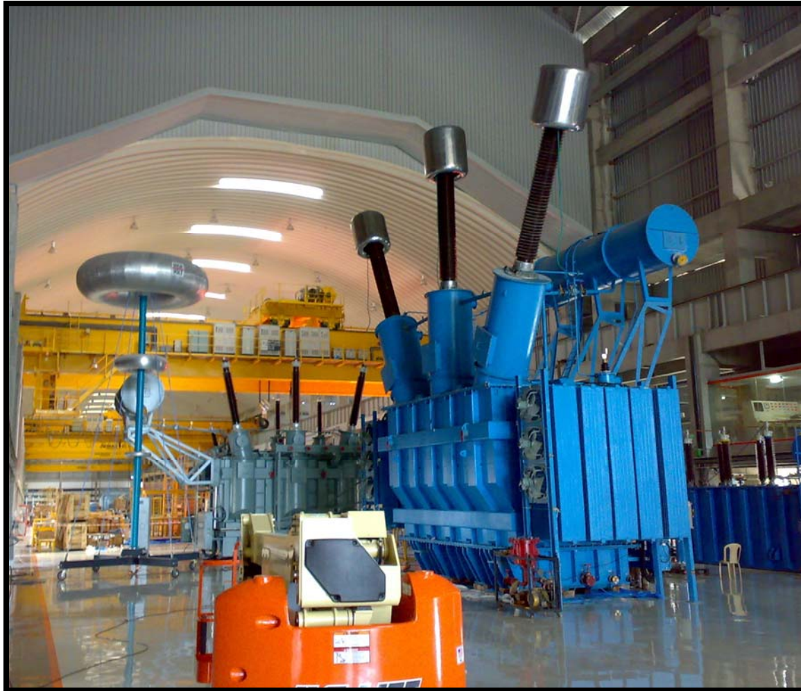
400 KV Transformer under testing at Moraiya plant
