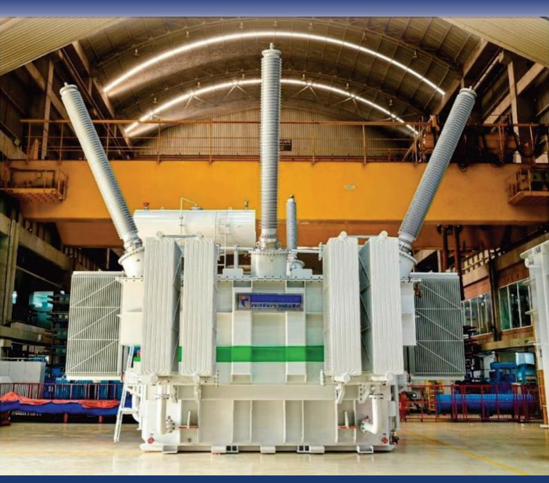
World's First 420kV Ester Fluid Filled Shunt Reactor
