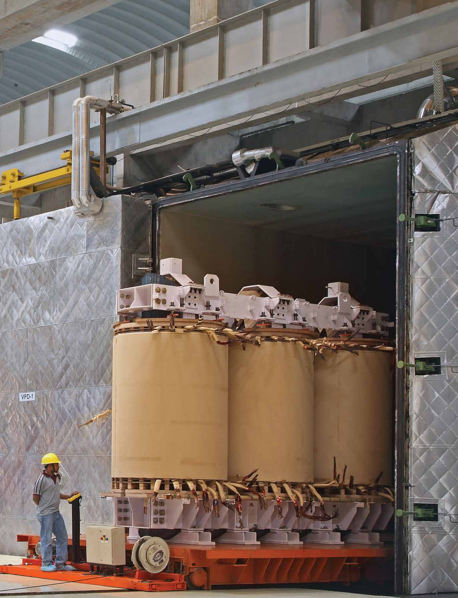
■ 5 indigenously developed Vapour Phase Drying Chambers to process Transformers upto 1200 kV Class
